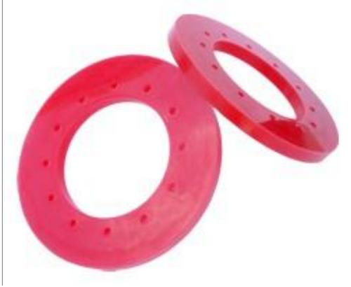
Standard scraper discs are constructed of high-grade abrasion and chemical resistant solid-cast polyurethane material. Sizes 2" through 14" are manufactured for center-rod-type pigs with center-hole, and sizes 16" through 48" are manufactured with bolting pattern configuration. Options include neoprene, viton, epdm, buna-n or other elastomer compounds for special services; varying durometers (hardness); customized dimensions for special pigging applications.
